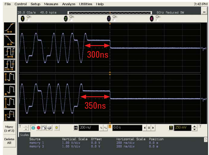
Figure 7. The TP_IDL is a positive-going pulse with a width of 300 ns or 350 ns depending on whether the last bit was one or zero respectively.
