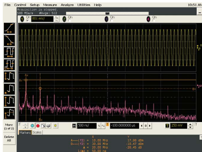
Figure 10. The oscilloscope display is divided into two, with the trace on the upper portion displaying the all-1's Manchester-encoded signal. The trace on the lower portion uses the oscilloscope FFT function to measure harmonic content of the all-1's Manchester-encoded signal. This example shows a marker at the fundamental frequency of 10 MHz and another marker on the third harmonic (30 MHz). The magnitude of the third harmonic shown here is -28.45 dB from the fundamental.
